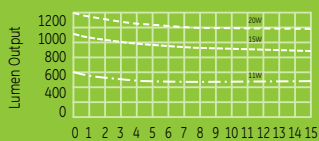
Lumen maintenance characteristics of Biax™ and Electronic Biax™ lamps
